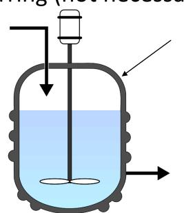
So when we are sizing a liquid CSTR, we mean what volume of the physical reactor is needed if it is filled up. (i.e., going from a 10 L to 20 L CSTR wouldn't change things if you still only have 10 L of liquid inside)
