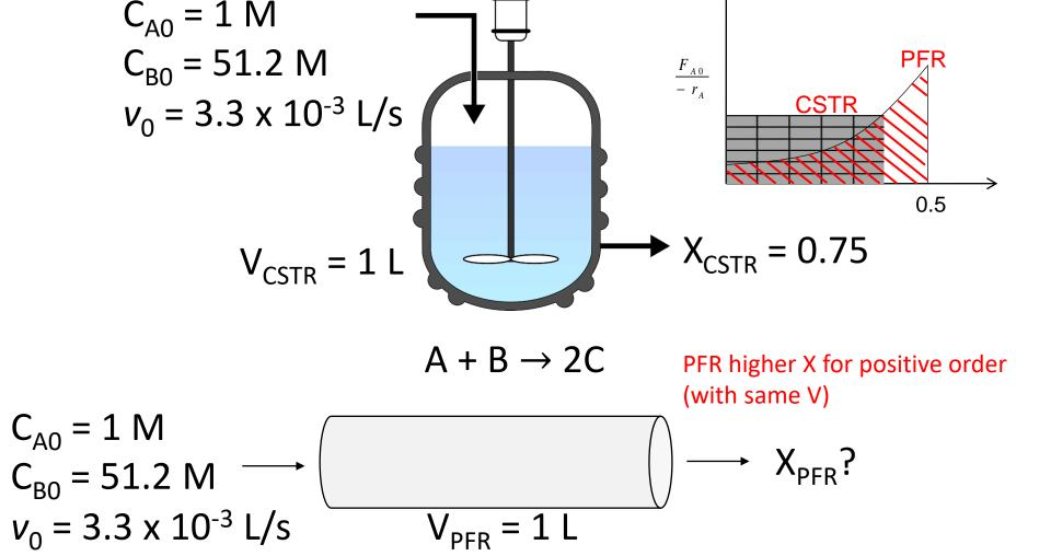
Now, the same liquid-phase reaction but in a plug flow reactor (PFR) instead of a CSTR.
